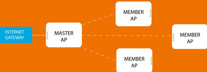
Uncomplicated network setup anyone can do in 10 minutes out of the box. You just configure one master AP using a setup wizard on your smartphone, and the master configures the rest for you, automatically.
