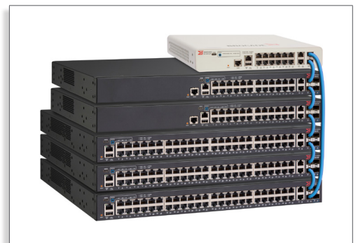
Figure 1: Stacking on standard Ethernet ports A stack of ICX 7150 showcasing the use of standard SFP+ 10Gbps dual-purpose ports and standard SFP+ short copper cables. The same ports can be used as 10GbE uplinks when not used for stacking.
