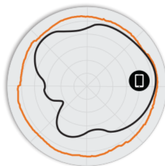
Figure 3. T610o 5GHz Azimuth Antenna Patterns
