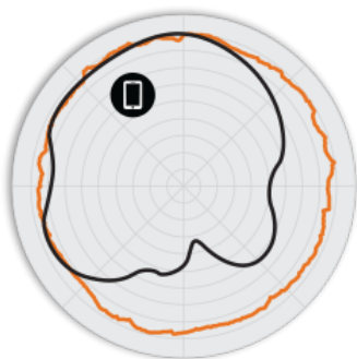
Figure 2. T610o 2.4GHz Azimuth Antenna Patterns
