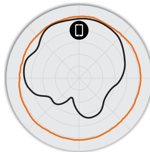
Figure 3. H500 5GHz Azimuth Antenna Patterns
