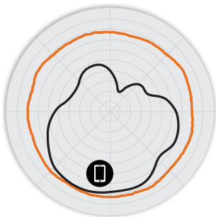
Figure 2. H500 2.4GHz Azimuth Antenna Patterns
