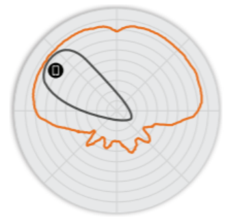
Figure 5. C110 5GHz Elevation Antenna Patterns
