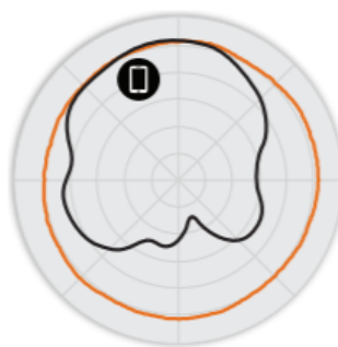
Figure 4. C110 2.4GHz Elevation Antenna Patterns
