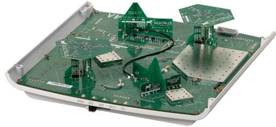
Patented smart antenna arrays in every access point provide longer range and more reliable Wi-Fi connections, requiring fewer APs than competitive alternatives.
