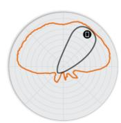
Figure 5. T811 5GHz Elevation Antenna Patterns
