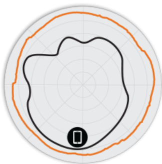
Figure 2. T811 2.4GHz Azimuth Antenna Patterns
