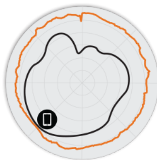
Figure 3. T811 5GHz Azimuth Antenna Patterns
