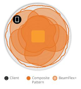
Figure 2. T811 2.4GHz Azimuth Antenna Patterns
