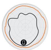
Figure 3. T811 5GHz Azimuth Antenna Patterns
