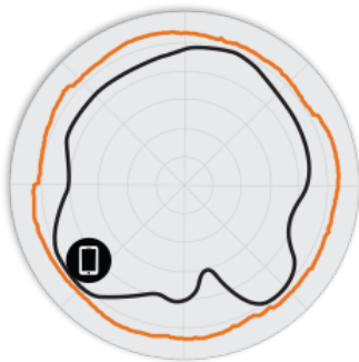
Figure 2. T305 2.4GHz Azimuth Antenna Patterns
