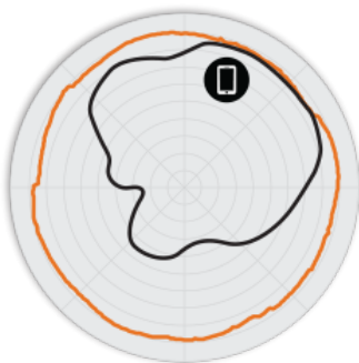
Figure 2. T301n 2.4GHz Azimuth Antenna Patterns
