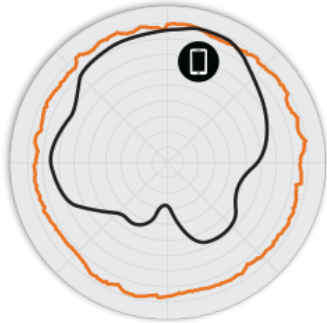
Figure 2. R750 2.4GHz AzimuthAntenna Patterns
