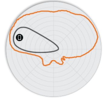
Figure 5. R750 5GHz Elevation Antenna Patterns
