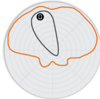
Figure 4. R750 2.4GHz Elevation Antenna Patterns
