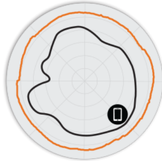
Figure 3. R750 5GHz AzimuthAntenna Patterns
