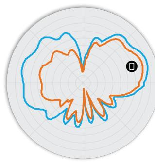
Figure 5. R730 5GHz ElevationAntenna Patterns
