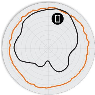
Figure 3. R730 5GHz AzimuthAntenna Patterns
