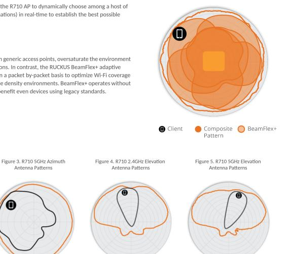
Note: The outer trace represents the composite RF footprint of all possible BeamFlex+ antenna patterns, while the inner trace represents one BeamFlex+ antenna pattern within the composite outer trace.
