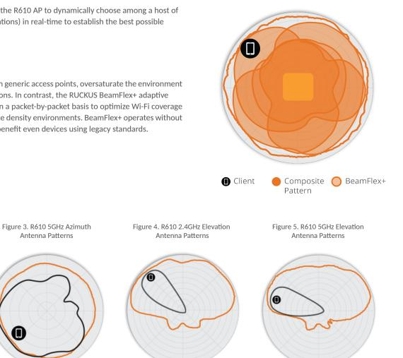
Note: The outer trace represents the composite RF footprint of all possible BeamFlex+ antenna patterns, while the inner trace represents one BeamFlex+ antenna pattern within the composite outer trace.
