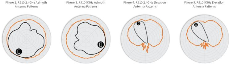
Note: The outer trace represents the composite RF footprint of all possible BeamFlex+ antenna patterns, while the inner trace represents one BeamFlex+ antenna pattern within the composite outer trace.
