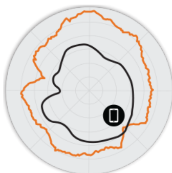
Figure 3. 7781-CM 5GHz Azimuth Antenna Patterns
