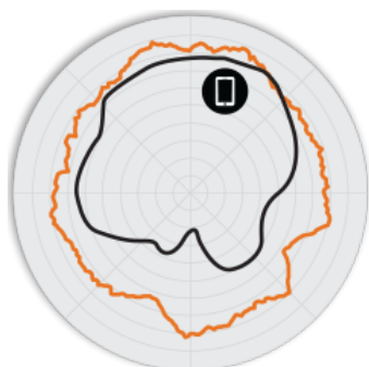
Figure 2. 7781-CM 2.4GHz Azimuth Antenna Patterns
